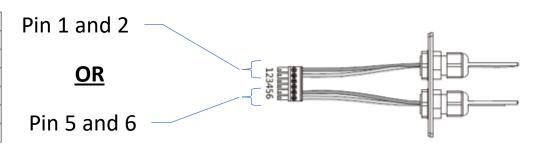
Pin 1/Pin 5 => Catch Solar Relay RS485 A Pin 2/Pin 6 => Catch Solar Relay RS485 B
