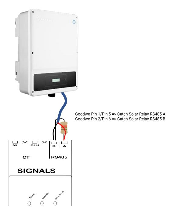
Ensure the data cable is rated for the voltages it will be in close proximity to. A 120 Ohm terminating resistor may be required at the CATCH Relay terminals as shown in the diagram below if the cable run is longer than 10m.
