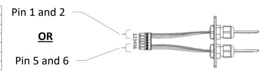
Pin 1 or Pin 5 => Catch Solar Relay RS485 A Pin 2 or Pin 6 => Catch Solar Relay RS485 B
