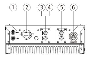
The image above is the bottom of the NS Series inverter.
